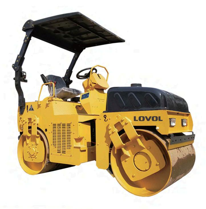
**ZB390B Engine Model** 26.5KW Rated Power 3500KG Operating mass
